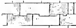
STONE CUTTING, FIG. 1: WITH JOGGLED JOINTS, GIVING GREAT SOLIDITY TO THE WORK; SYRIA, 4TH CENTURY.
